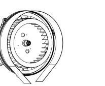
**5.** Clean flywheel, mesh strip, and the inner and outer housing of dust. Replace the flywheel and tighten driveshaft nut.
