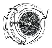
**3.** Release the mesh strip. WARNING: Careful to not let the mesh spring open which can cause injury.
