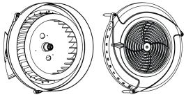
**4.** Using the 17mm wrench, undo the flywheel driveshaft nut and remove the flywheel.
