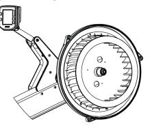
**6.** Insert the mesh strip into the slot in the inner housing overlapping the mesh at the bottom.
