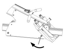
**6.** Test the movement of the front assembly along the rails. It should move freely along the rails but tight enough to have a stable connection to the rails. Make small adjustments to tighten or loosen the roller tension.
