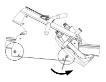
**2.** Locate the adjuster bolts on the underside of the front assembly. Insert the 4mm allen key into the socket of the rear adjuster bolt and while holding steady in position, use the 13mm end of the 13mm/16mm wrench to loosen in a **clockwise** direction, the roller adjuster locking nut about a 1/2 turn.
