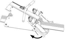
**7.** Lock the rear roller adjuster by inserting and holding the 4mm key in a steady position in the adjuster bolt. If the adjuster bolt turns while tightening it will alter the adjustment. Using the 13mm wrench, tighten the locking nut in an **anticlockwise** direction.
