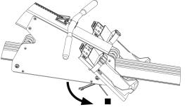
**9.** Test row the DX after adjustment and adjust tuning again if necessary. Finally, tighten the axle side bolts on both side of the front assembly.
