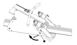
**4.** Using just the 4mm key, loosen both front and rear rollers in an **anticlockwise** direction until the front assembly moves loosely along the rails.
